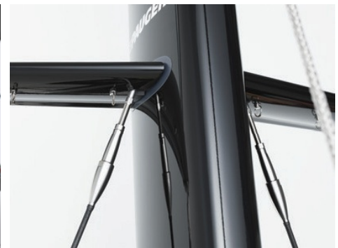
Examples of stainless-steel fittings to carbon rigging.
