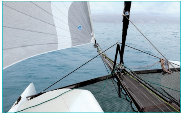
This bowsprit is rated for a breaking moment of thirty tons, which is about nine times more than is needed.
