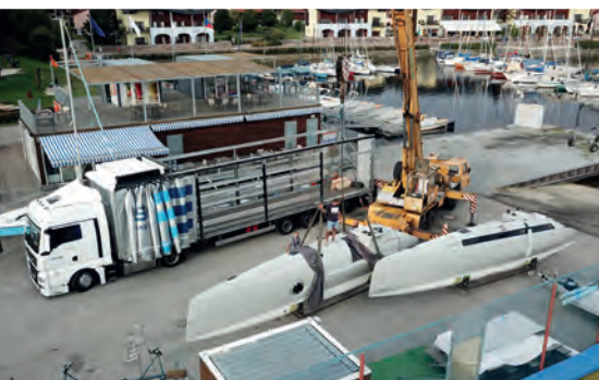
The IC36 is dismantlable and transportable - it can travel by truck or in a 40-foot shipping container.
